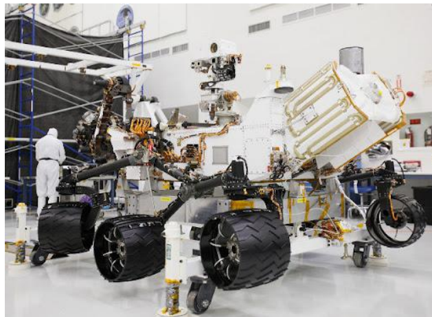
Figure 6. Curiosity Rover Radioisotope Thermoelectric Generator
