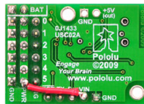
Micro Maestro configured to use a single power supply for both board and servos.
